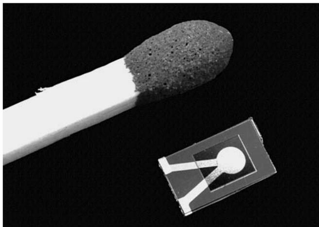
**Fig. 4** A quartz crystal resonator coated with two gold electrodes that are then coated with a chemical linker layer and a receptor or cell. This device is then integrated into either a cuvette or a flow cell for delivery and removal of ligands, etc.
