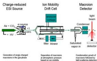
Schematic representation of the ion flow path (TSI Inc.)
